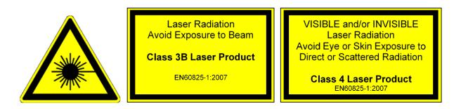
Z-Laser declares the conformity to a laser safety class according to EN ISO 60825-1 only for the complete product entity. Whenever this entity is changed the laser safety class is voided.
