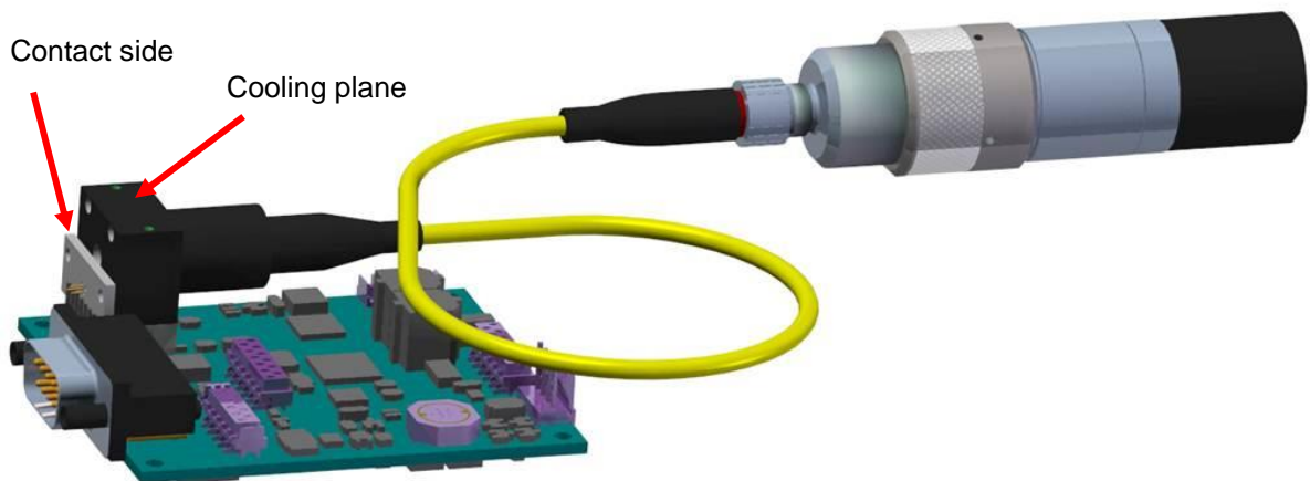
Picture 2 An active, or very good passive, cooling capability must be provided and attached to the marked cooling plane. Any sort of condensation must be prevented though. Attention: prevent to expose the contact side of the laser diode to any sort of mechanical stress. Otherwise suffer severe damages and malfunction are likely to occur.
