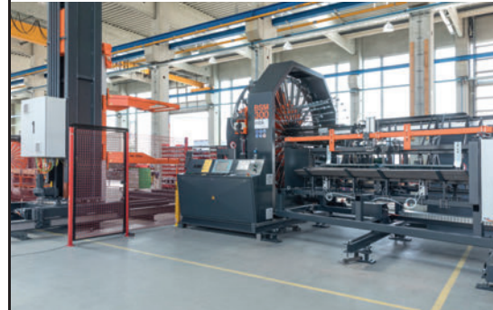
Cage welding machines for manhole and concrete pipe reinforcements
