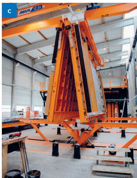
Fig. 9c-e: Two Abus indoor cranes, each with a load capacity of 12.5 tonnes, lift the prepared butterfly formwork until the backs of the two formwork panels touch (the prepared formwork panels face outwards).
