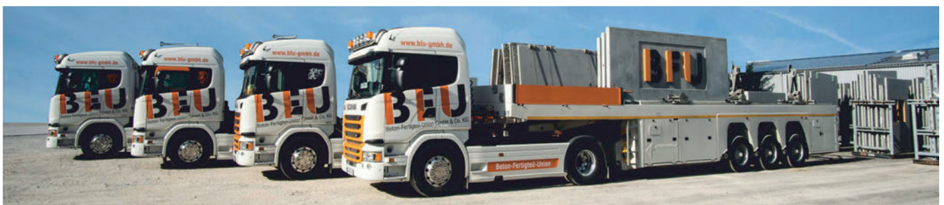
Fig. 12: Ready for transport - with BFU's own trucks and inloaders from Faymonville, the high-quality, fair-faced precast concrete elements reach the construction sites in the southern German state of Baden-Württemberg and in neighbouring Switzerland.
