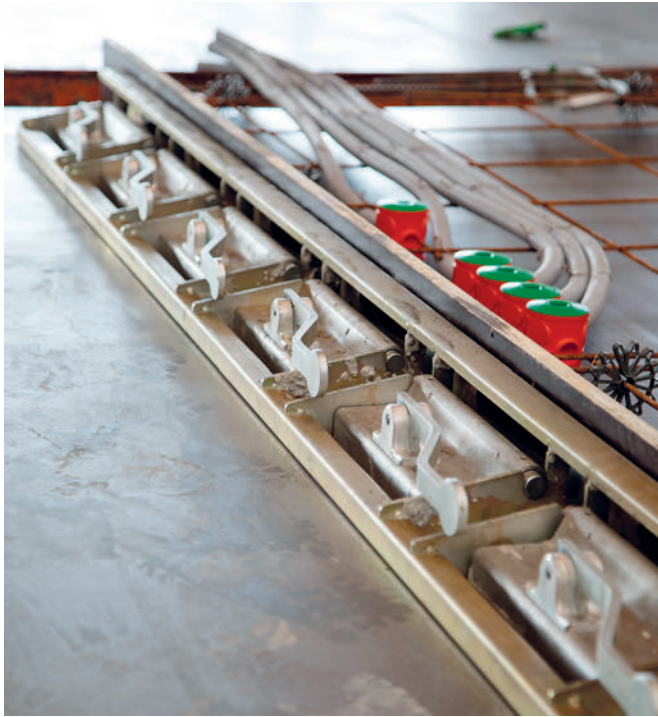
Fig. 8: For use in production at the manufacturer Beton-Fertigteil-Union, the profile of the MultiForm formwork beam was adapted and reinforced; it was also designed so that more MagFly magnets can be placed at smaller distances from each other. The shuttering can thus withstand high pressure when concreting vertically in the butterfly battery mould.
