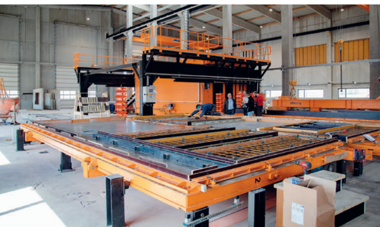
Fig. 1: German precast producer BFU successfully commissioned the new butterfly battery mould with butterfly formwork from BT innovation at his production site in Schramberg-Waldmössingen at the beginning of 2021.
