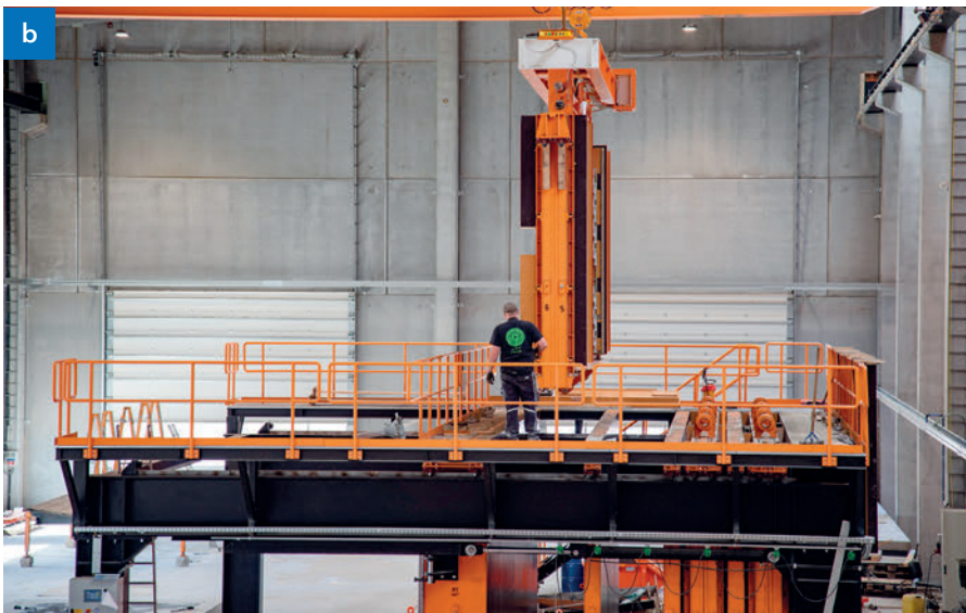
Fig. 10a+b: Hovering and positioning of the closed, prepared butterfly formwork above the battery mould. In the middle of the upper photo, directly next to the battery mould, the maximally extended, orange-coloured arms of the device for opening or closing the butterfly formwork can be seen.
