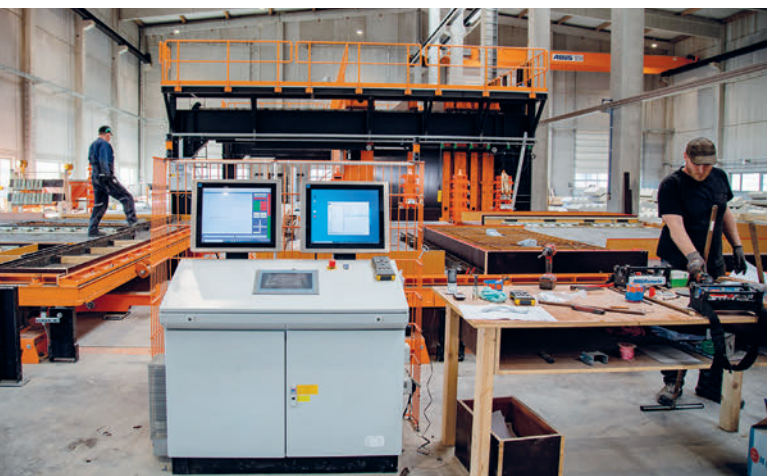
Fig. 6: The control panel for the two work stations, with a butterfly formwork each lying open (immediately to the left and right behind it) and the side view of the battery mould in the background – the battery mould has its own control panel.
