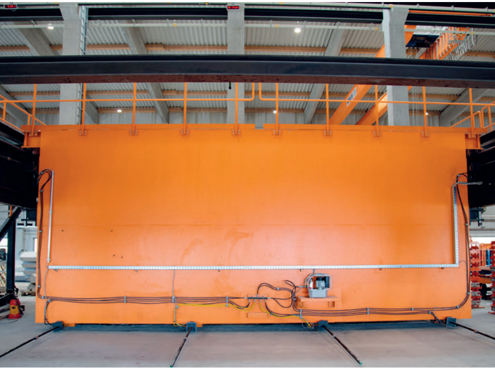
Fig. 4: Frontal view of the still unclad, movable tension wall of the butterfly battery mould; four hydraulic cylinders on the lower, longer edge of the tension wall ...
